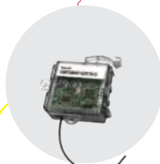
Two hardwired outputs GATE MODULE 806SA-0040 RS485
